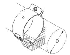
HF-cable clamp for fastening to profile rails
