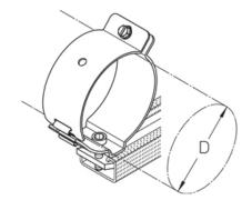
HF-cable clamp for fastening to profile rails
