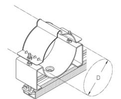
HF-cable clamp for fastening to profile rails
