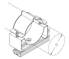
HF-cable clamp for fastening to profile rails
