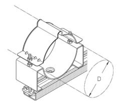
HF-cable clamp for fastening to profile rails
