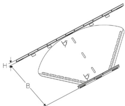
cable tray bend, variable, height = 35 mm
