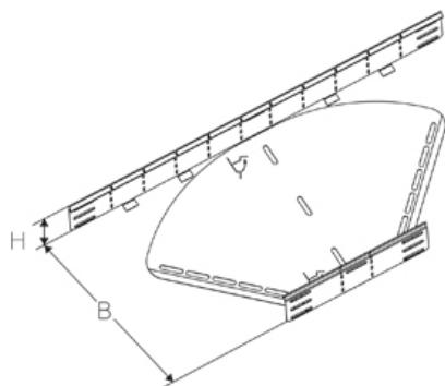
cable tray bend, variable, height = 85 mm
