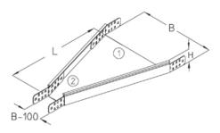
cable tray reducer, height = 35 mm
