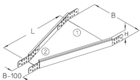
cable tray reducer, height = 35 mm
