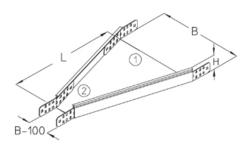
cable tray reducer, height = 85 mm
