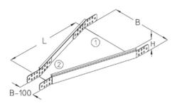
cable tray reducer, height = 85 mm
