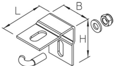
storm protection angle - mesh cable tray
