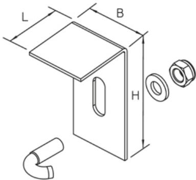
storm protection angle - mesh cable tray
