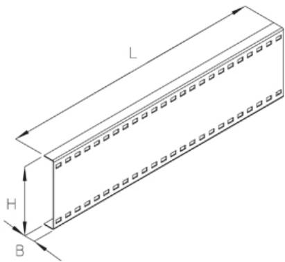
wide-span connector, height = 200 mm
