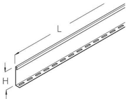
wide-span separating strip, height = 50 mm
