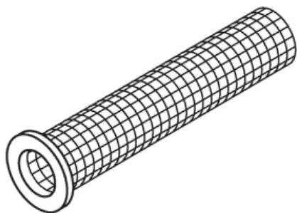
perforated bush for shear connector, stone
