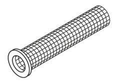
perforated bush for shear connector, stone
