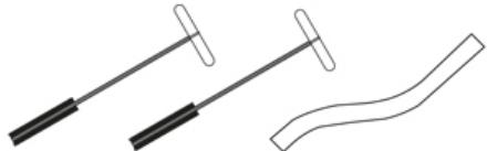
shear connector rod, brush
