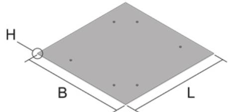
Steel sheet as an optional accessory for the temporary covering of a mounting opening in hollow floors or screed floors caused by the removal of a shuttering unit or plastic formworks. (Diameter: 307 mm and 261x261 mm) With press-in threaded bolt to prevent slipping.
