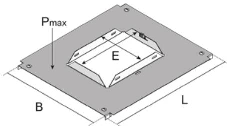
Assembly covers made of Sendzimir hot-dip galvanized sheet steel for latching to the side profile of the bottom part of the cable duct including turning bolt. Usable as pull- and installation box, with one opening for insertion of a shuttering unit that will be replaced with a rectangular assembly unit during final assembly.
