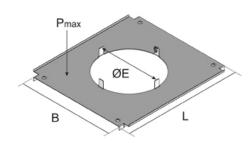
cable duct assembly cover, double, round
