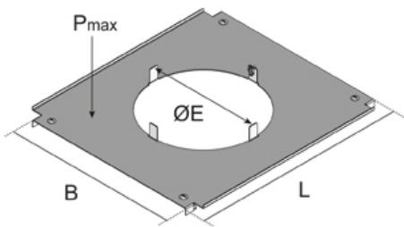
cable duct assembly cover, double, round
