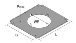
cable duct assembly cover, double, round
