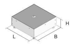
heat resistant shuttering unit, levellable, angular
