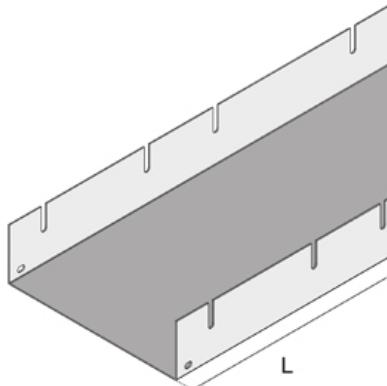
Screed-flush heavy-duty duct made of Sendzimir hot-dip galvanized sheet steel as open duct bottom piece for horizontal leading of cables, with slots as retainers for side profiles.
