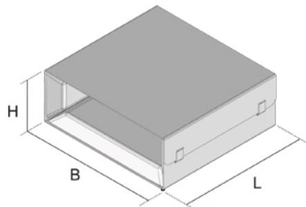
Duct fire protection partition as a four-sided S30/S90 folding box for the installation in an existing wall opening (H = 90 mm, W = 180 mm). For lightweight and solid walls from 100 mm thickness.
