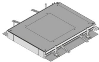
Attachment assembly cover set, triple, made of sheet steel, pre-assembled on aluminum side profile with bolted traverse, pre-punched dummy assembly opening and end piece. Designed for office traffic loads.
