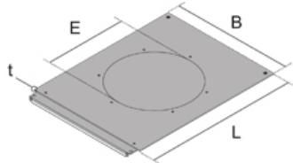
Assembly dummy cover with round opening made of Sendzimir-hot-dip-galvanised steel sheet. To be used in replacement for a dummy cover for the accommodation of one installation unit, double. Designed for office traffic loads.
