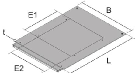
Assembly dummy cover with square opening made of Sendzimir-hot-dip-galvanised steel sheet. To be used in replacement for a dummy cover for the accommodation of one installation unit, triple. Designed for office traffic loads.
