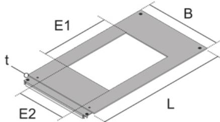
Assembly cover with square opening made of sendzimir hot-dip galvanised steel sheet. Can be used instead of a dummy cover to accommodate a double installation unit. Designed for office traffic loads.
