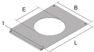
Assembly cover with round opening made of sendzimir hot-dip galvanised steel sheet. Can be used instead of a dummy cover to accommodate a double installation unit. Designed for office traffic loads.
