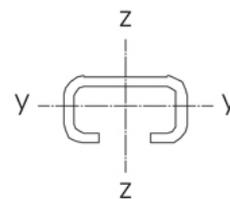
$$\begin{aligned}W_y &= 0.29 \text{ cm}^3 \\W_z &= 0.80 \text{ cm}^3 \\I_y &= 0.21 \text{ cm}^4 \\I_z &= 1.12 \text{ cm}^4\end{aligned}$$
