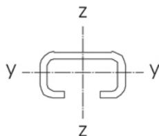
$$\begin{aligned}W_y &= 0.46 \text{ cm}^3 \\W_z &= 1.05 \text{ cm}^3 \\I_y &= 0.41 \text{ cm}^4 \\I_z &= 1.47 \text{ cm}^4\end{aligned}$$
