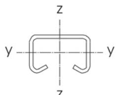
$$\begin{aligned} W_y &= 2.45 \text{ cm}^3 \\ W_z &= 5.42 \text{ cm}^3 \\ l_y &= 4.33 \text{ cm}^4 \\ l_z &= 13.54 \text{ cm}^4 \end{aligned}$$
