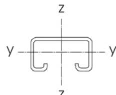
$$\begin{aligned} W_y &= 1.76 \text{ cm}^3 \\ W_z &= 3.85 \text{ cm}^3 \\ l_y &= 2.64 \text{ cm}^4 \\ l_z &= 9.23 \text{ cm}^4 \end{aligned}$$
