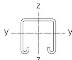
$$\begin{aligned} W_y &= 3.19 \text{ cm}^3 \\ W_z &= 4.50 \text{ cm}^3 \\ l_y &= 7.31 \text{ cm}^4 \\ l_z &= 9.22 \text{ cm}^4 \end{aligned}$$
