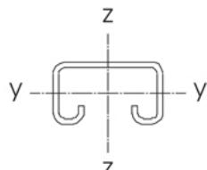
$$\begin{aligned} W_y &= 0.90 \text{ cm}^3 \\ W_z &= 1.75 \text{ cm}^3 \\ l_y &= 1.10 \text{ cm}^4 \\ l_z &= 3.46 \text{ cm}^4 \end{aligned}$$
