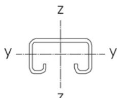
$$\begin{aligned} W_y &= 1.10 \text{ cm}^3 \\ W_z &= 2.25 \text{ cm}^3 \\ l_y &= 1.34 \text{ cm}^4 \\ l_z &= 4.32 \text{ cm}^4 \end{aligned}$$
