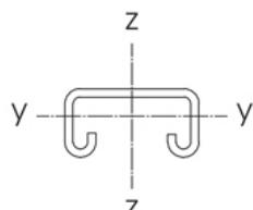
$$\begin{aligned} W_y &= 0.92 \text{ cm}^3 \\ W_z &= 2.56 \text{ cm}^3 \\ l_y &= 1.02 \text{ cm}^4 \\ l_z &= 5.25 \text{ cm}^4 \end{aligned}$$
