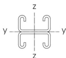
$$\begin{aligned} W_y &= 2.80 \text{ cm}^3 \\ W_z &= 5.12 \text{ cm}^3 \\ l_y &= 5.87 \text{ cm}^4 \\ l_z &= 10.50 \text{ cm}^4 \end{aligned}$$
