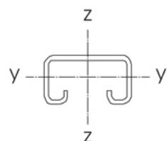
$$\begin{aligned}W_y &= 1.05 \text{ cm}^3 \\W_z &= 2.24 \text{ cm}^3 \\l_y &= 1.18 \text{ cm}^4 \\l_z &= 4.48 \text{ cm}^4\end{aligned}$$
