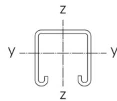
$$\begin{aligned}W_y &= 2.01 \text{ cm}^3 \\W_z &= 2.91 \text{ cm}^3 \\l_y &= 4.19 \text{ cm}^4 \\l_z &= 5.96 \text{ cm}^4\end{aligned}$$
