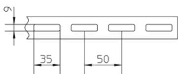
$$\begin{aligned}W_y &= 0.30 \text{ cm}^3 \\W_z &= 0.83 \text{ cm}^3 \\l_y &= 0.25 \text{ cm}^4 \\l_z &= 1.25 \text{ cm}^4\end{aligned}$$
